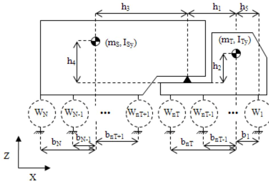
Figure 1(b) Side view sketch of Tractor + Trailer.
