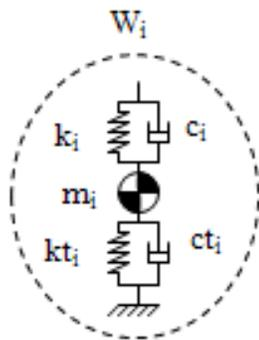
Figure 1(a) Suspension and tyre system.
