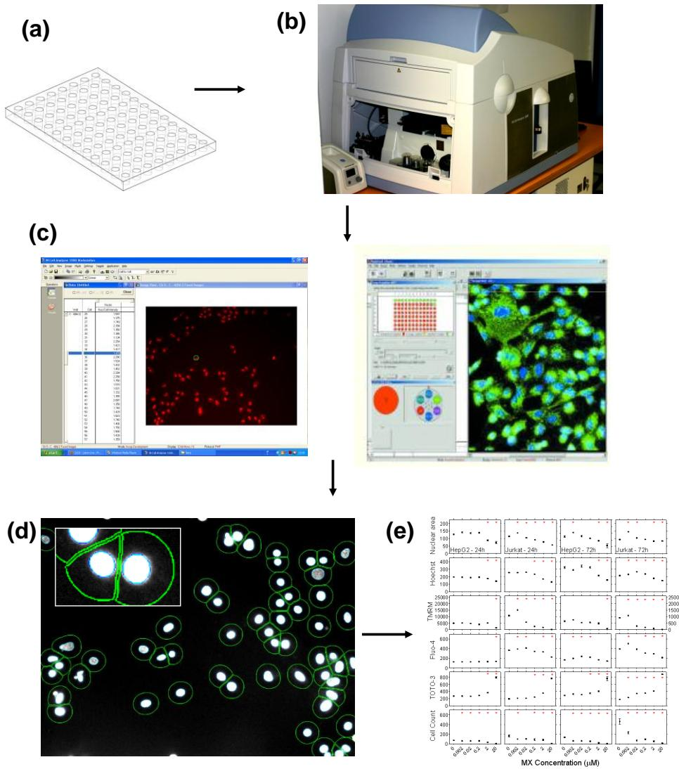
**Fig. 1:** Schematic representation of HCA. Instrumentation exploits the combined power of high throughput multi-well automation with epifluorescence microscopy as well as the capability of multi-wavelength fluorescent dye analysis. (a) Cells treated in multiwell plates and stained with fluorescent dye cocktail, (b) plate is docked in the live cell
