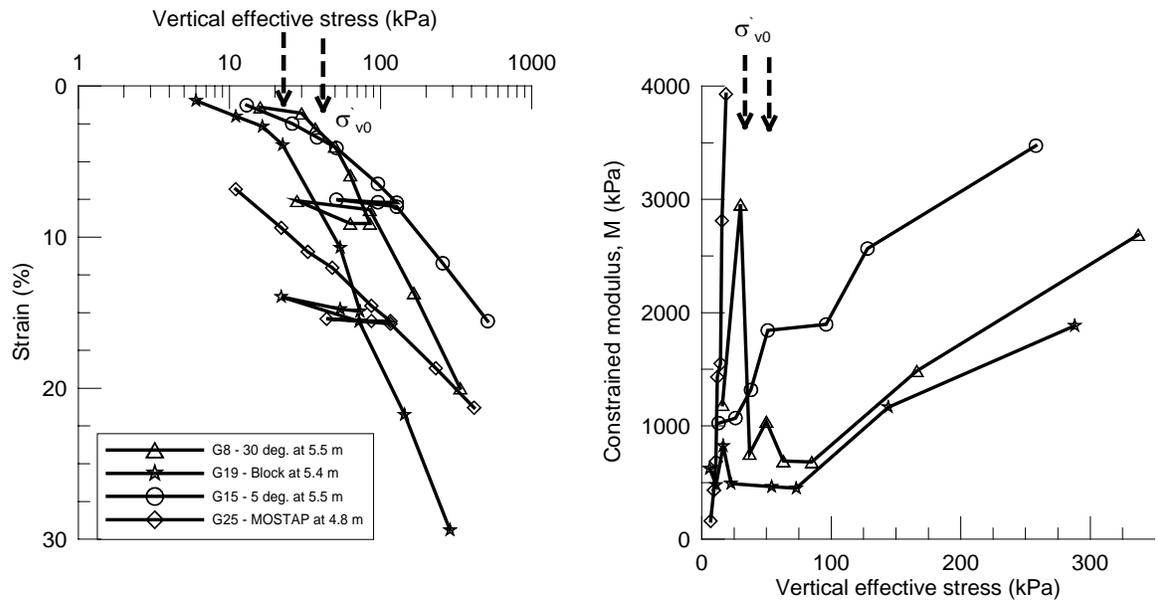
Figure 12. Results of IL oedometer tests
