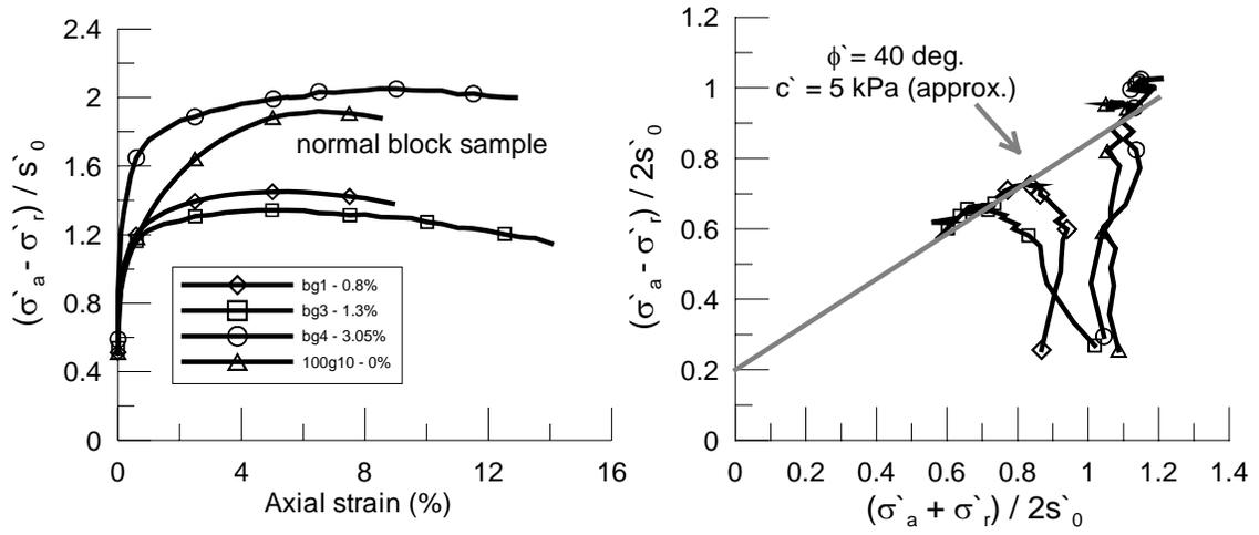
Figure 11. Results of ISA tests on block samples
