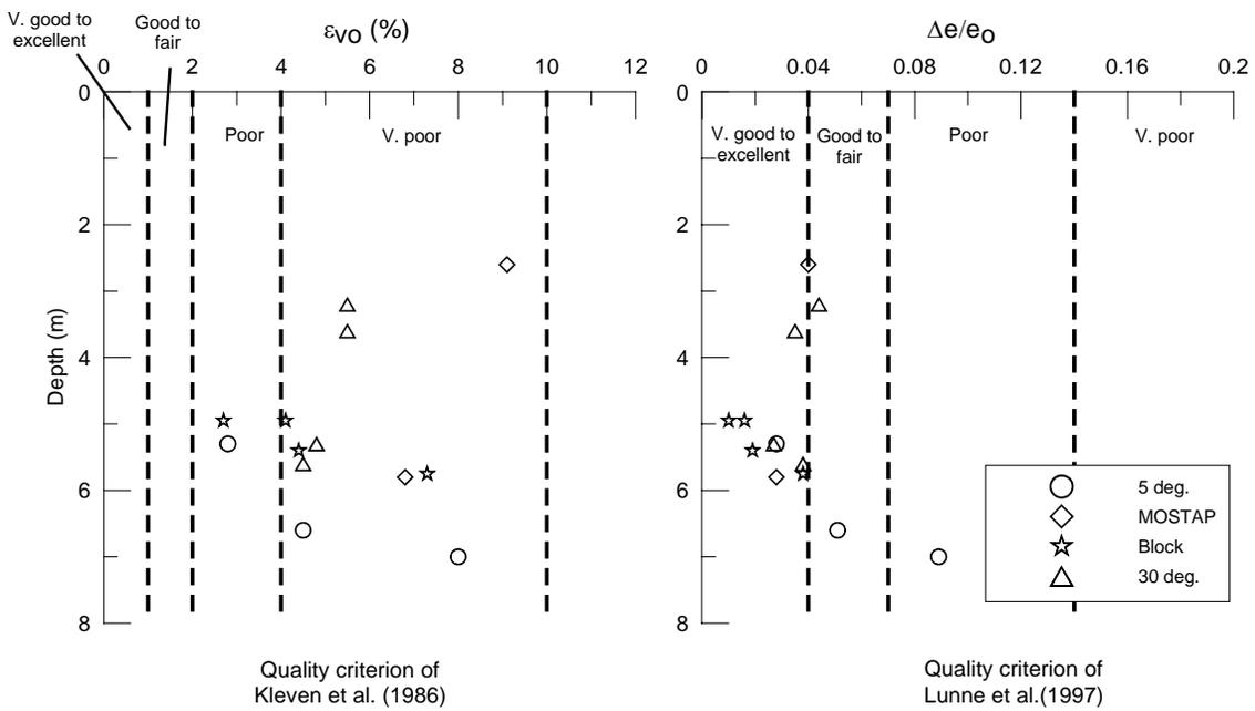
**Figure 8. Assessment of sample quality – triaxial tests**
