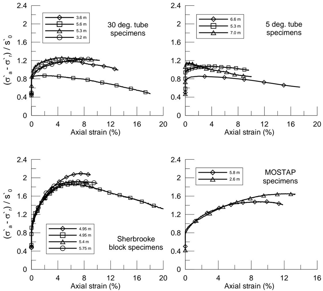
**Figure 9. CAUC test deviator stress – strain plots**
