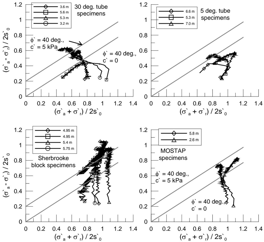
**Figure 10. CAUC test – stress path plots**
