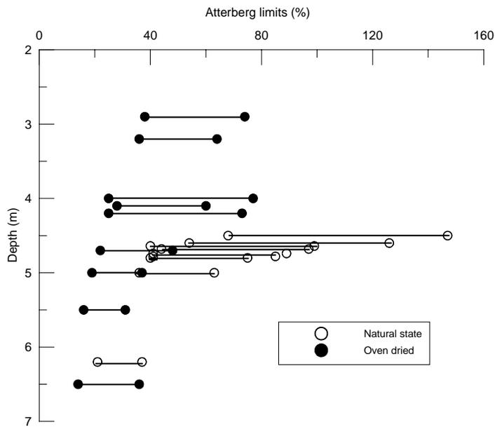
**Figure 6. Influence of oven drying on Atterberg limits**
