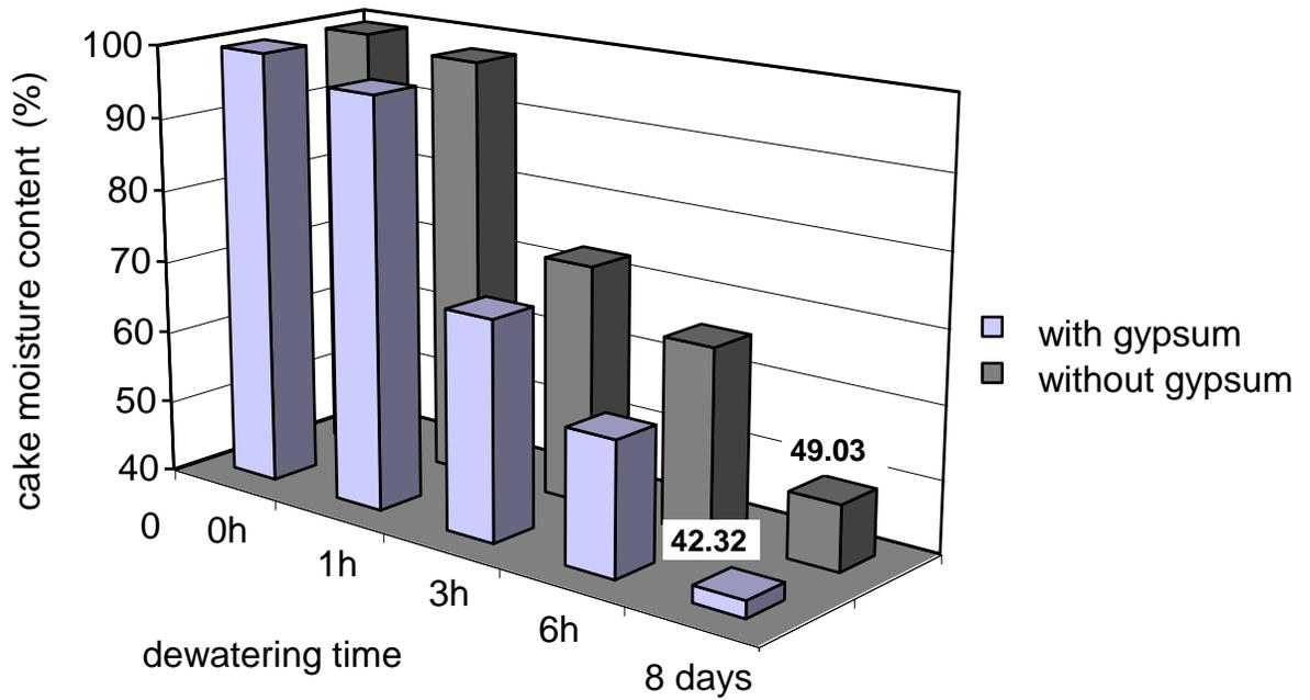
Fig. 4 Identification of dewatering behaviour with or without gypsum addition at applied pressure of 5.0 bar in air pressure plate (polymer dose of 20.0 mg/l, numeric values representing the cake equilibrium moisture content).
