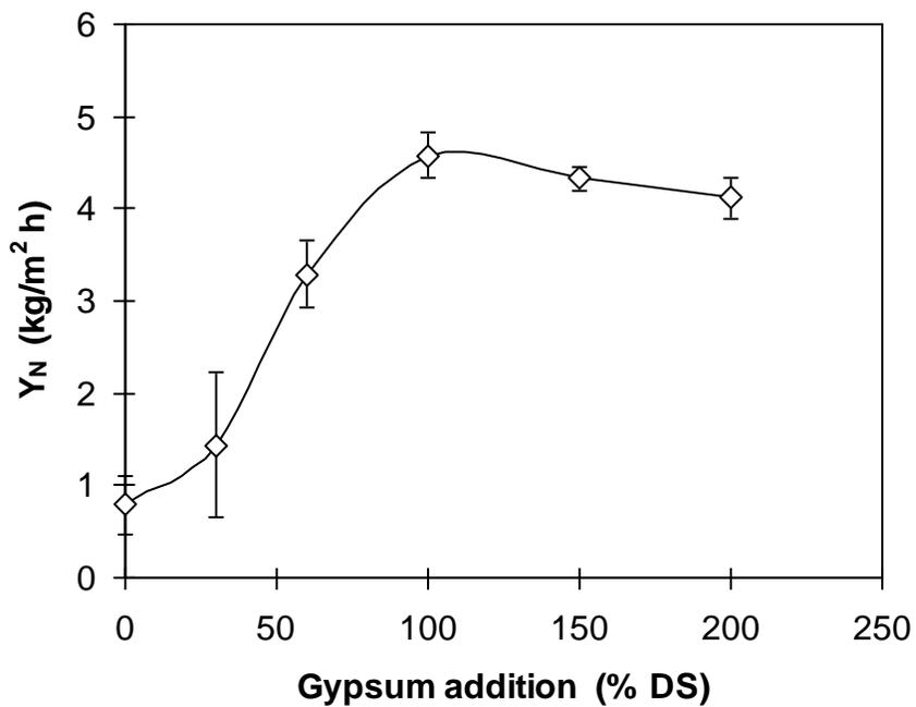
Fig. 2 filterability as a function of gypsum addition (% DS, referring original sludge dry solids) during conditioning at polymer dose of 20.0 mg/l (error bars denote SDs).
