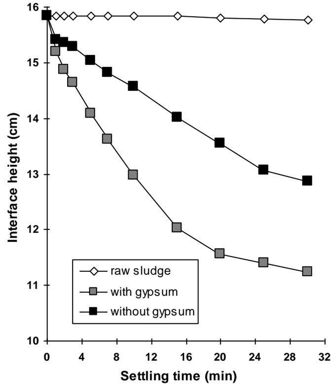
Fig. 5 Settling behaviour of raw and conditioned sludge with or without gypsum addition in a 100 ml measuring cylinder (sludge solids concentration of 9230 mg/l, polymer dose of 20.0 mg/l, gypsum addition of 100 % DS).
