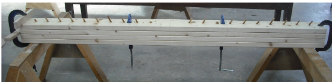
Fig. 5: Four-layer beam held in clamps during construction
