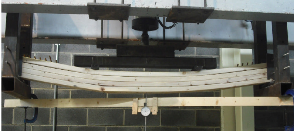
Fig. 10: Four – layer 44-dowel beam at failure
