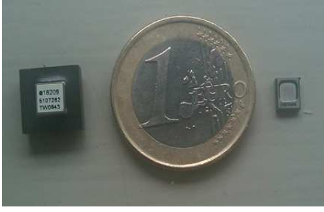
Figure 2: Form factor of IMU (left) and ultrasonic receiver (right) used in the sensor units
