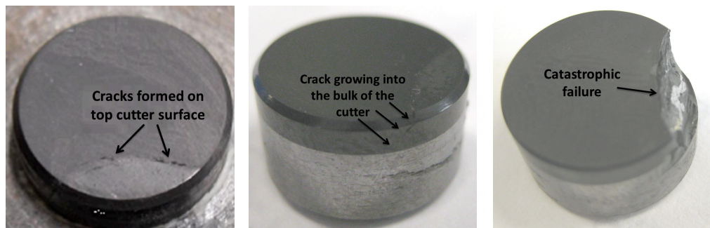
Figure 5: Failure of the PDC cutter under cyclic impact loading, showing the (a) initial stage, (b) intermediate stage where the crack has extended by more than 2mm into the diamond layer thickness and (c) final stage (catastrophic failure).
