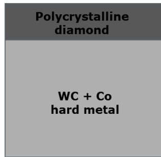
Figure 1: Geometry of a typical PDC cutting tool used in Oil & Gas drilling.
