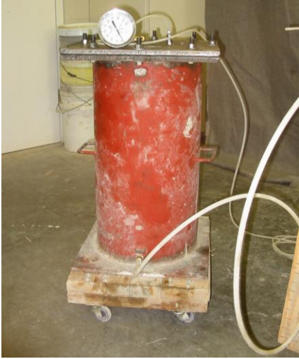
Figure 2: Pressurized Grout Tank
