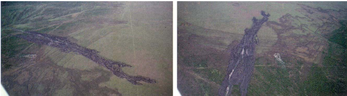
Figure 16. Peat slide in Slieve Bloom Mountains, Co. Laois, 1988. Note run out distance and scars of old slides.
