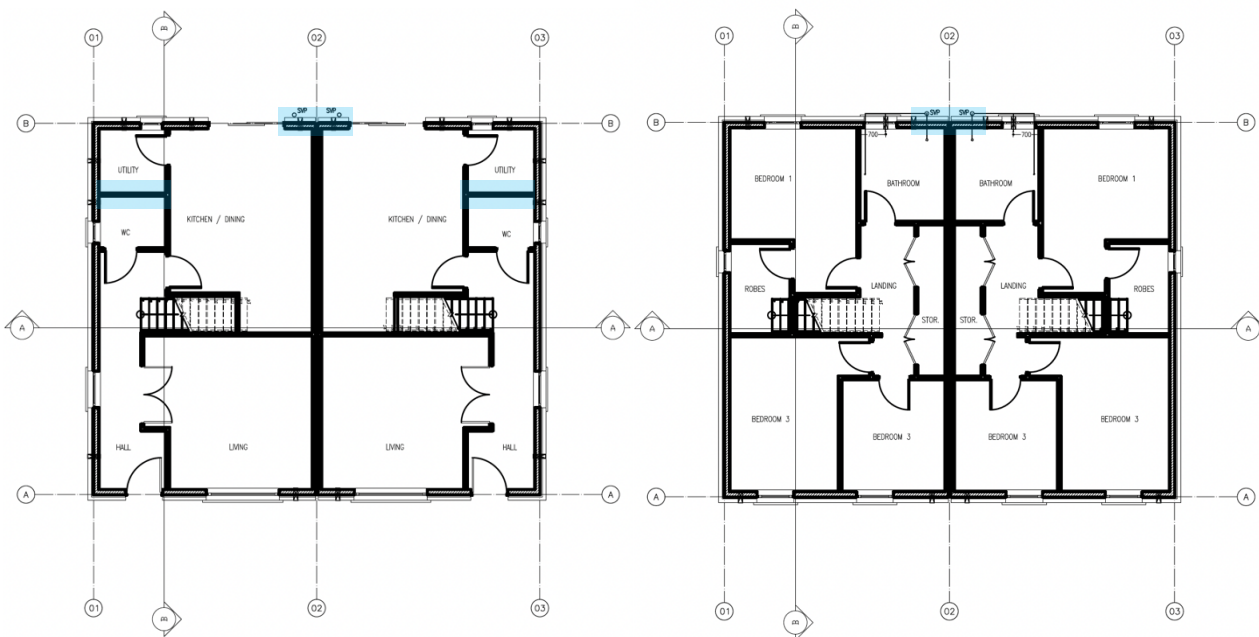
Figure 3.1: Ground Floor (left) and First Floor plans of semi-detached houses (blue highlights water and plumbing) (Cygnum)
