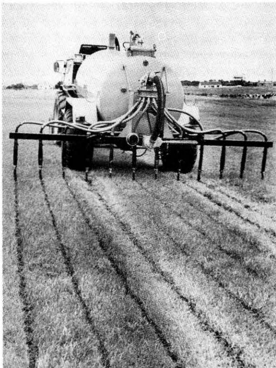
The bandspreader minimises drifting of slurry spray
