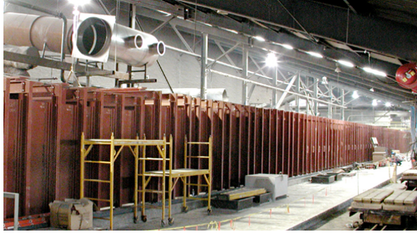
Fig. 9. Modern Tunnel Kiln (GGB 2003)
