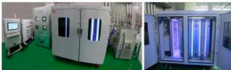
Figure 9: Image of photochemical skid. Reprinted with permission from [72]. Copyright (2020) American Chemical Society.
