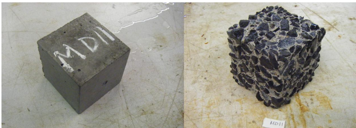
Fig. 7. Effect of acid exposure on cube samples (cube shown corresponds to 100% CEM I)
